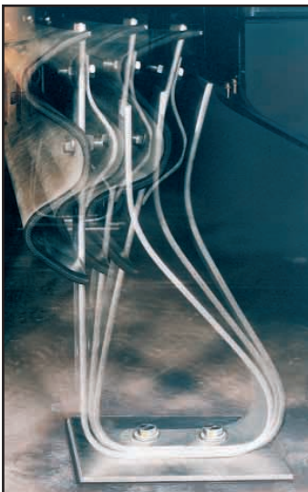
Spring Steel Buffers deflecting under impact
